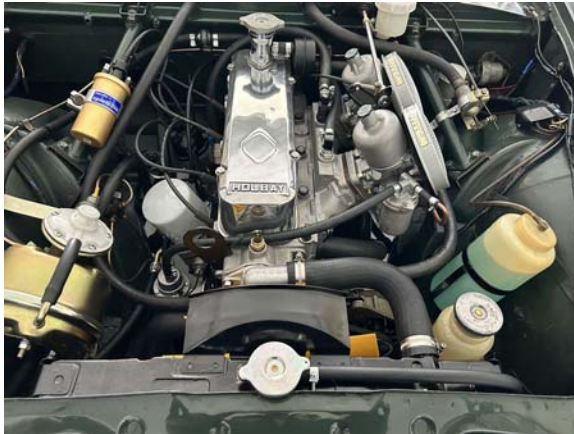
Engine layout . Note the use of Volvo P1800 S radiator overflow tank and early original windscreen washer reservoir
